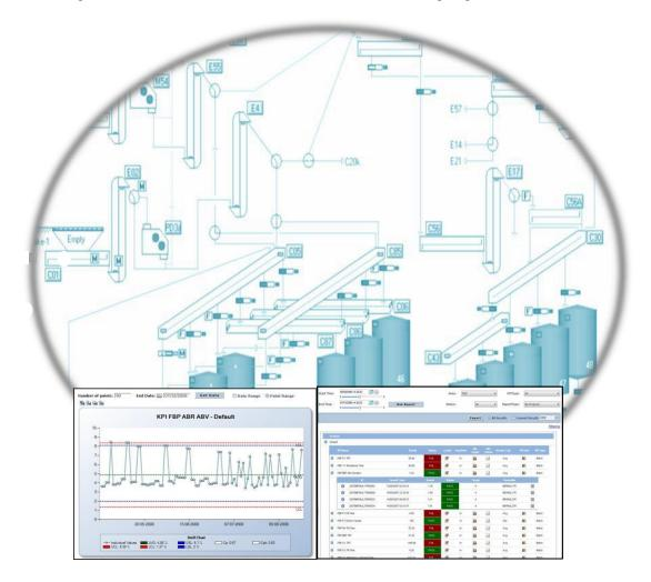
The system links the brewery's control system directly to SAP to enable condition and counter based monitoring of plant. This functionality will enable the automation of Preventative Maintenance Orders and has allowed the maintenance teams to move away from the traditionally time based PMOs thus prioritizing resources.
